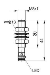
Inductive Sensors BES 516-343-G-E5-C-S 49 M8x1 x 44 normally-open Sn=2mm shielded
